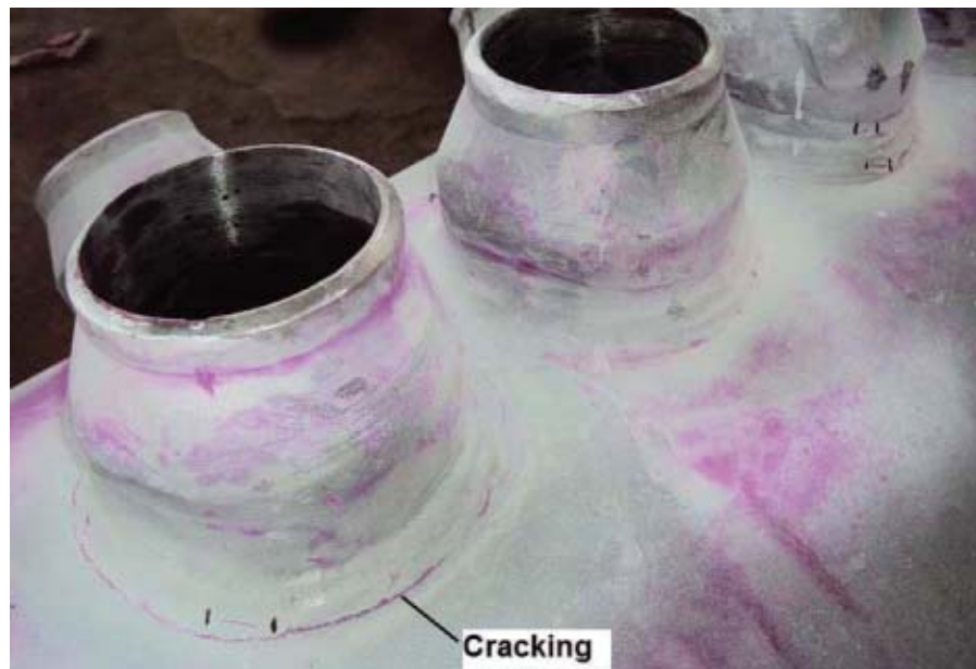
Fig. 1 — Stress relief cracking in a 321 stainless steel heat exchanger header.
