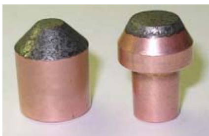
Fig. 4 — Coated weld electrodes are able to provide a hard wear surface as well as a barrier between the copper electrode and the zinc steel coating.
