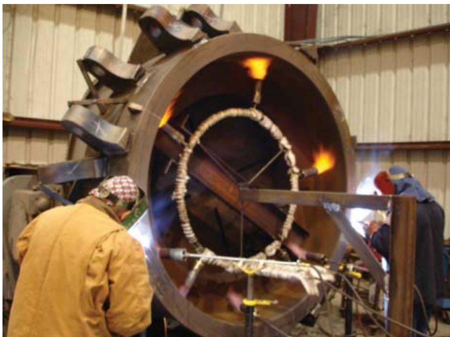
Continuous welding of 4-in.-thick 4130 pad eyes to a 4130 ring, maintaining a 450°F pre-heat for 12 days.
