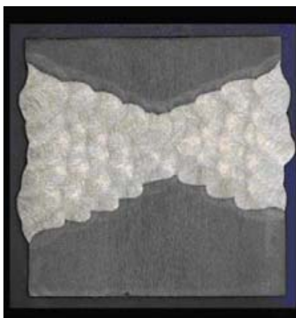
Fig. 1 — A 2-in.-thick weld made by T-GMAW in the horizontal (2G) position.
