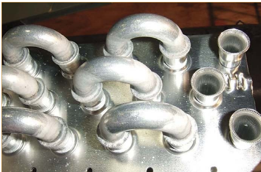
Fig. 1 — Air-conditioning coils are one example of a high-volume assembly currently manufactured out of aluminum.
