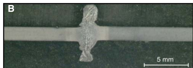
Fig. 2 — High-frequency welds made in advanced high-strength steels (different composition than the DP600 but still possessing near 600 MPa ultimate tensile strength). A — As-welded specimens; B — transverse micrograph. Previously published in Ref. 6. Used with permission from US Steel Research Europe, Kosice, Slovak Republic.
