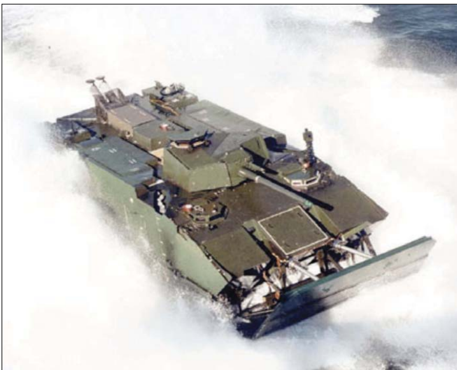
Fig. 6 — The advanced amphibious assault vehicle (AAAV) uses welded aluminum to produce a lightweight, high-speed vehicle that is effective on land and water.
