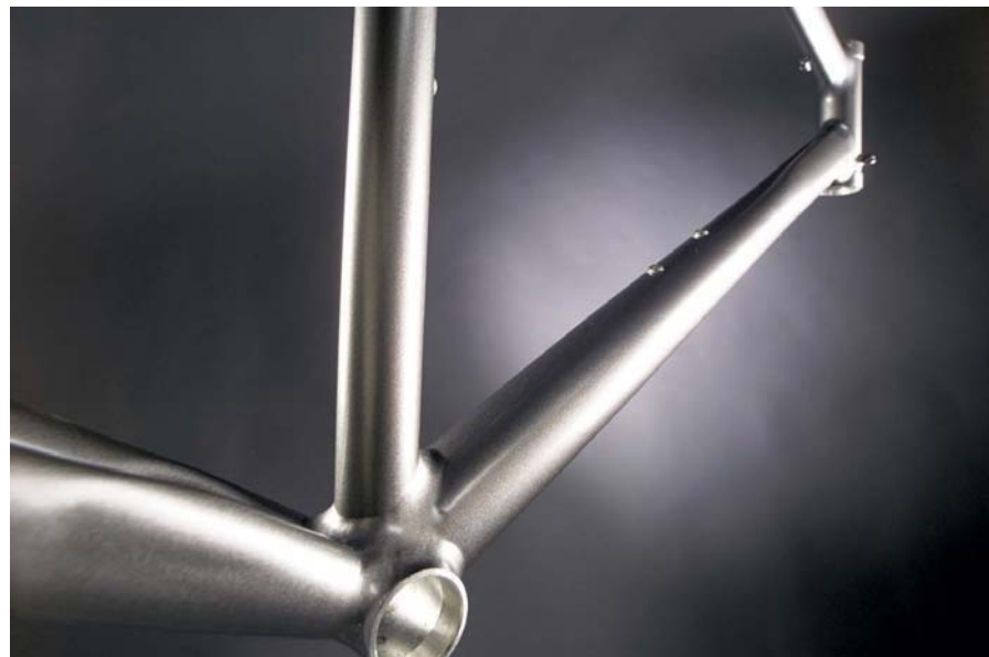
Fig. 4 — Aluminum bicycle frame manufactured from heat-treatable aluminum base metal. Welded with a heat-treatable aluminum filler alloy and subjected to postweld heat treatment in order to return the aluminum alloy to its original unwelded strength. (Photo courtesy of Cannondale.)
