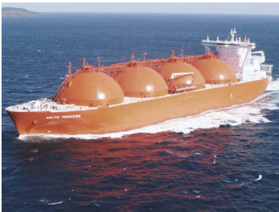
Fig. 5 — Liquefied natural gas (LNG) tanker with four large welded aluminum spheres (tanks). Many materials when subjected to these very low temperatures undergo changes in their physical structure that severely limit their usefulness in cryogenic applications. Some metals, for example many steels, become extremely brittle. Aluminum alloys, however, have been demonstrated to have an unusual ability to maintain their ductility and resistance to shock loading at extremely low temperatures approaching absolute zero -459^{\circ}\text{F} ( -273^{\circ}\text{C} ). As temperature decreases below room temperature, aluminum's tensile and yield strengths actually increase as the temperature decreases, and the ductility and toughness of most alloys increase as well. Even at the lowest test temperatures available, in liquid helium at -452^{\circ}\text{F} ( -273^{\circ}\text{C} ), strength remains high and ductility and toughness remain well above values for most alloys at room temperature.
