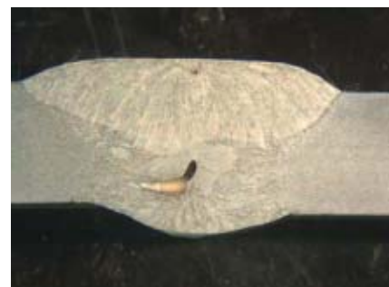
Fig. 2 — Porosity is most commonly caused by the presence of moisture in the weld.
