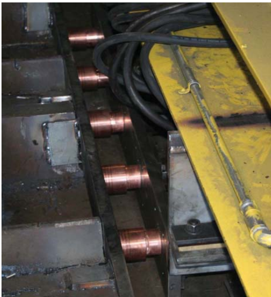
This 5000-A capacity sliding workpiece lead connection system enables fast travel speeds, cuts down on rework, and saves labor.
