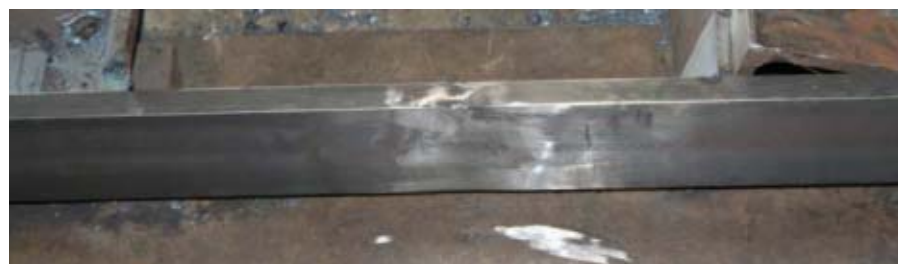
Fig. 3 — Between the individual bar lengths, each butt joint weld was buffed smooth.
