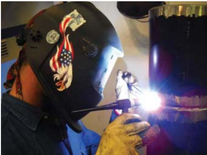
As part of his training at Energy Solutions Group, David Sanders performs gas tungsten arc welding on 6-in. pipe.
