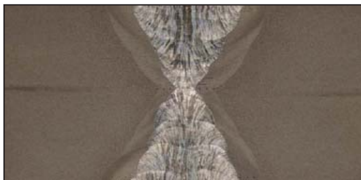
Fig. 3 — Macrograph of the welded joint.
