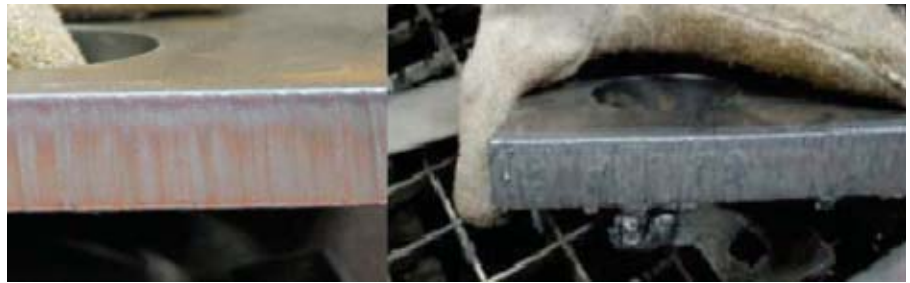
Plasma cut metal (left) is virtually dross-free compared with oxyfuel cut metal on right.
