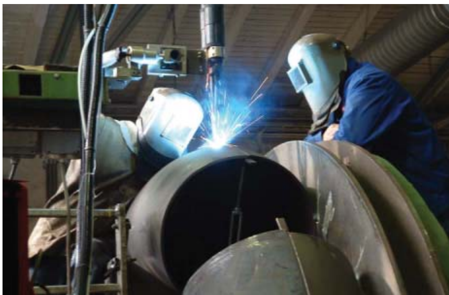
Fig. 5 — Welders at Uhlig Rohrbogen achieve a deposition rate that is up to 2.5 times faster when using the tandem wire system in comparison to single-wire welding.
