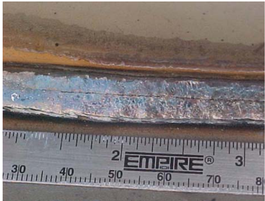
Fig. 2 — The centerline crack shown on this fillet weld is the result of low melting point material segregation (segregation cracking).
