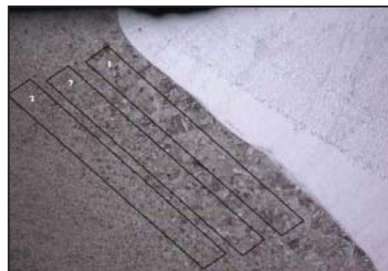
Fig. 4 — Microstructure of the different zones of the HAZ, which includes the situation of the extracted samples.
