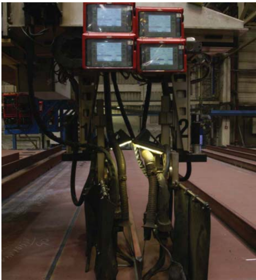
Fig. 4 — Two tandem systems — one on the right and one on the left — make the fillet weld joining the reinforcement plate and the floor area.
