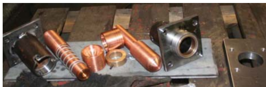
Fig. 2 — Various components make up the complete plunger.
