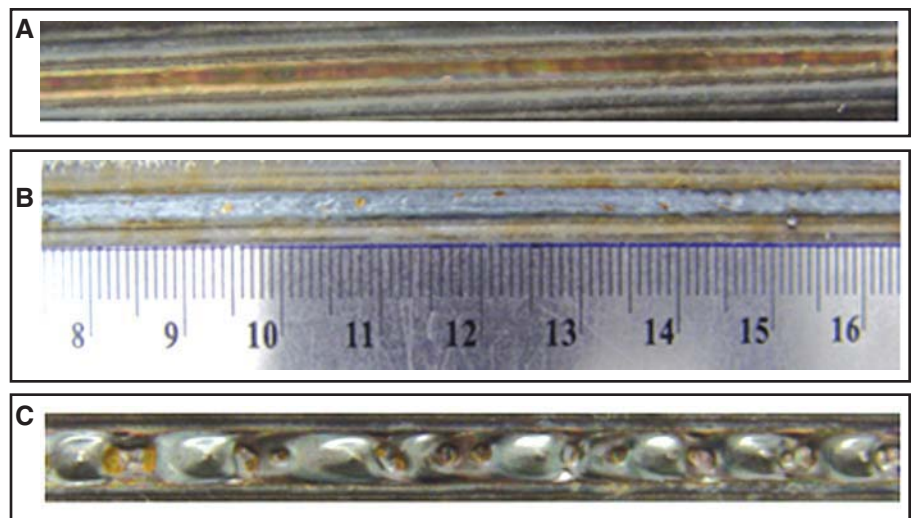
Fig. 16 — A — Top view of the preheating weld with the iron oxide film at the arc current of 230 A; B — top view of hybrid GTAW preheating/ laser welding with a separated molten pool; C — the humping produced in the GTAW preheating weld at an arc current of 240 A (welding speed: 30 mm/s; distance between the electrode tip and the top surface of two metal sheets: 3 mm; shielding gas flow rate: 30 ft 3 /h).
