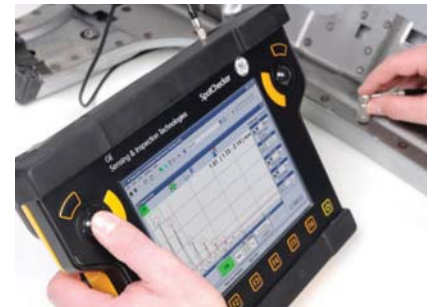
Fig. 3 — Instruments such as this Spotchecker™ ultrasonic spot weld inspection tool offer portability and easy-to-read screens.
