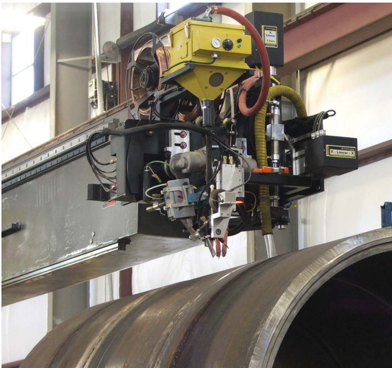
Fig. 2 — Welding equipment is usually suspended from a guide rail for outside welding.
