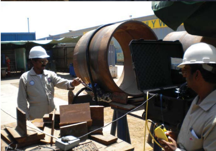
For codes permitting automated ultrasonic testing, inspectors may use hand-held (displayed at top) as well as motorized versions.
