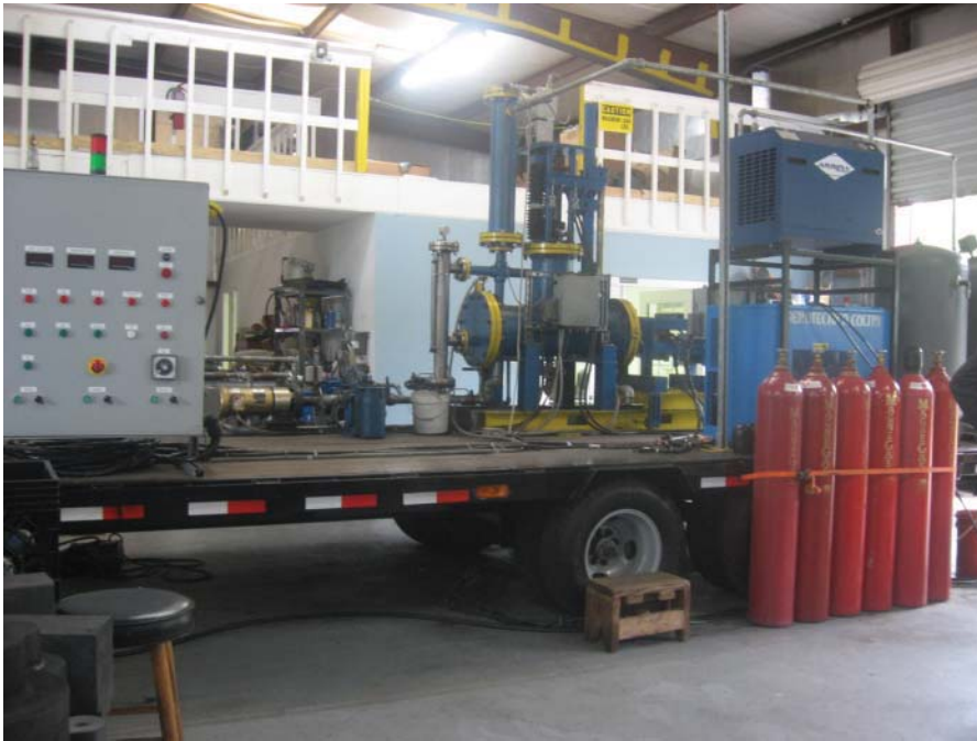
Fig. 4 — At the company's Florida production site, this machine makes fuel for distribution. Its control panel (left) is followed by the recycler (center) and high-pressure cylinders holding the end fuel product (right). Sludge from the City of Dunedin provides its feedstock.
