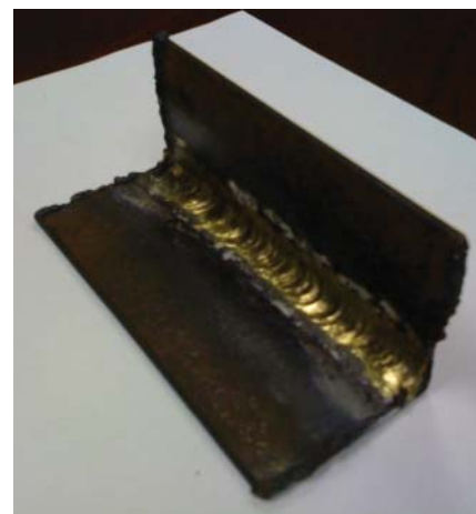
Fig. 3 — Result of a bronze brazing application showing this technology replaces acetylene for metal working industries.
