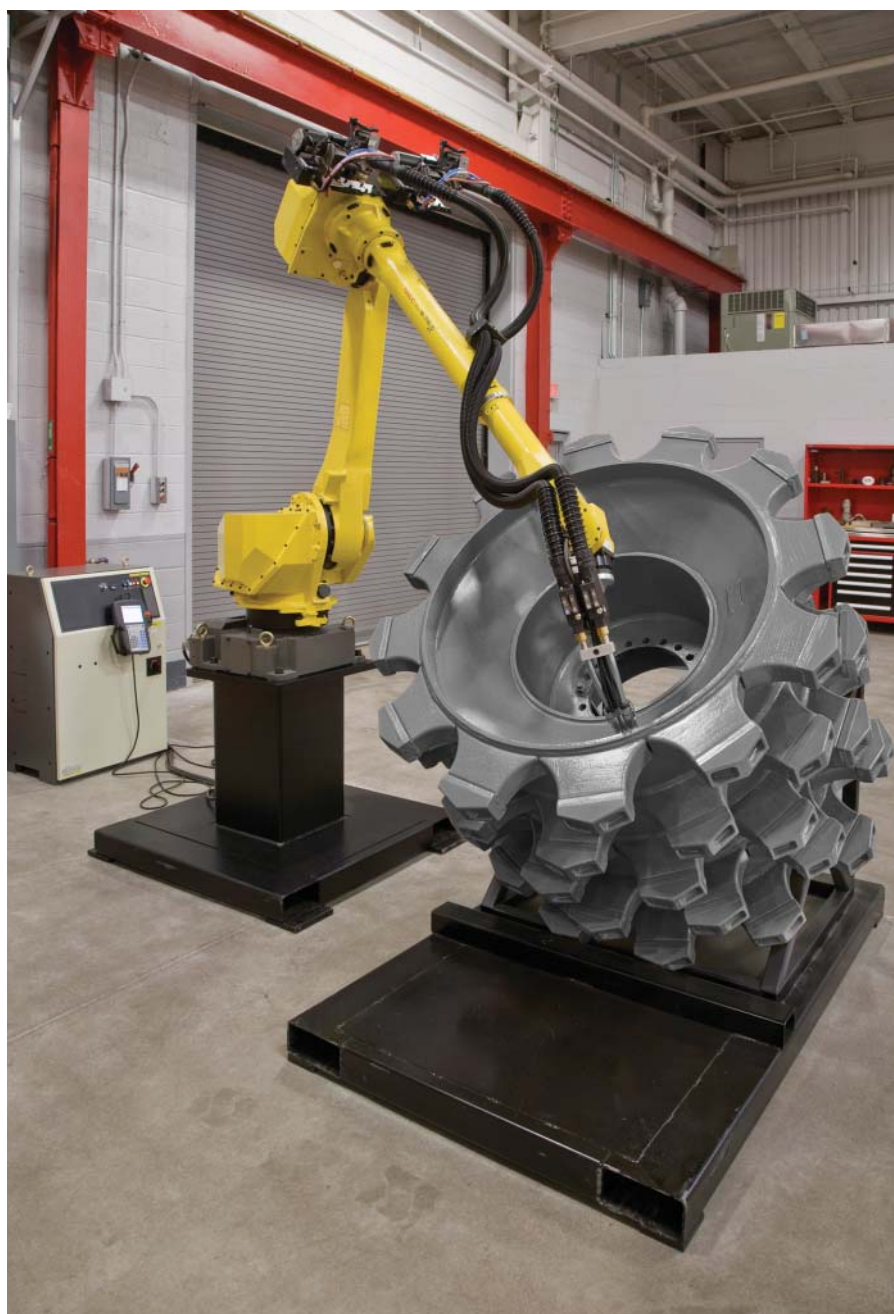
Fig. 2 — A FANUC Robotics M-710iC robot welds large, heavy compactor wheels. When welding very large parts such as a wind tower, fabricators need a larger welding robot with a longer reach such as this one.
