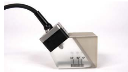
Fig. 2 — This new array fulfills all specifications to the American Welding Society's D1.1, Structural Welding Code — Steel.
