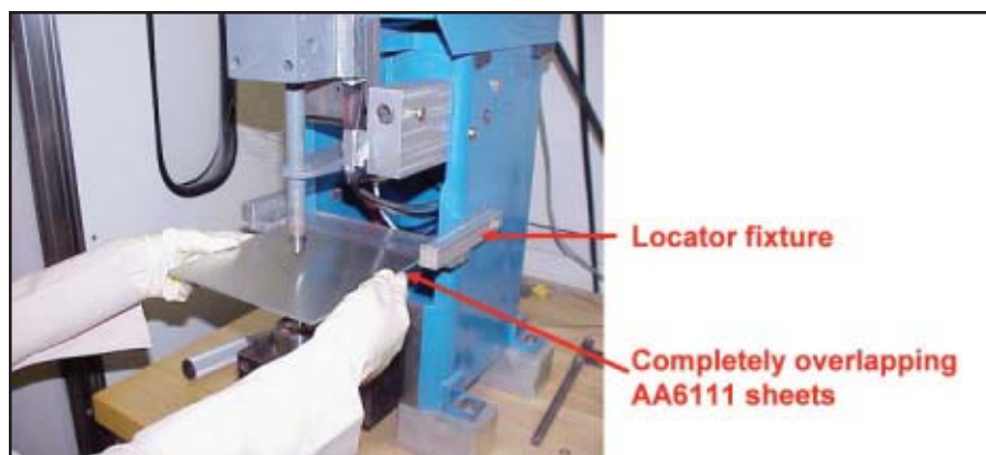
Fig. 2 — Welding setup for weld orientation and sheet rolling direction experiments.
