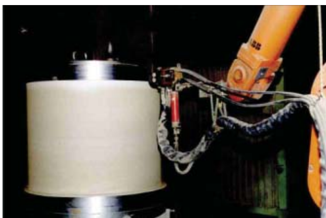
Fig. 9 — Bearing shaft with a Babbitt coating.
