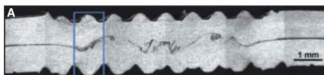
Fig. 10 — Ultrasonic weld microstructure as a function of cut direction: A — Cross section taken parallel to vibration direction; B — cross section taken perpendicular to vibration direction.
