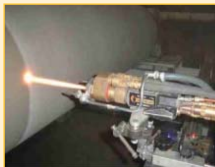
Fig. 1 — HVOF spraying of nano- and near-nano based materials.
