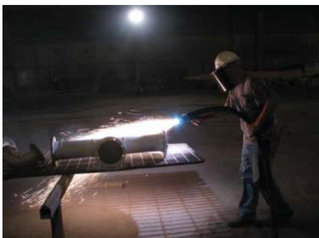
Fig. 7 — Arc spraying a T-joint with aluminum, 300 \mu m (12 mil).
