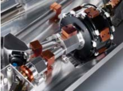
The layout of the disk laser technology that is being used to weld parts for the new Peugeot 3008.
