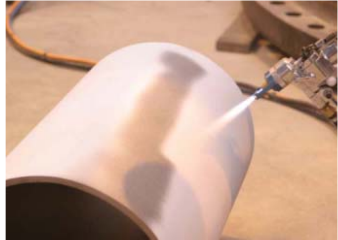
Fig. 3 — A pipe section undergoes flame spraying. (Courtesy of Metallisation Ltd., Dudley, England, Steve Barker.)
