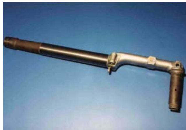
Fig. 6 — Nose gear of an F5 Tiger with a WC/CoCr coating.
