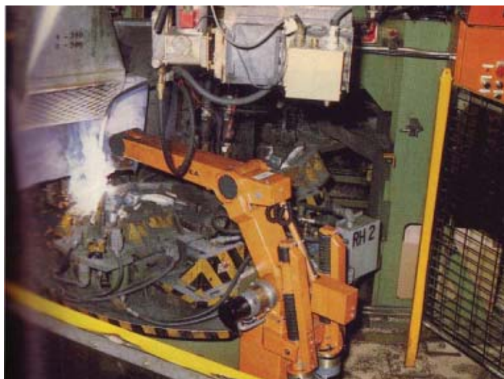
Fig. 9 — A robotic arc welding station custom designed to produce an automotive front crossmember assembly. The 1980s saw much greater use of arc welding robots in the United States. (Photo from the article titled “Speed Doubled on Robotic Arc Welding of Complicated Automotive Assembly” in the November 1986 Welding Journal.)
