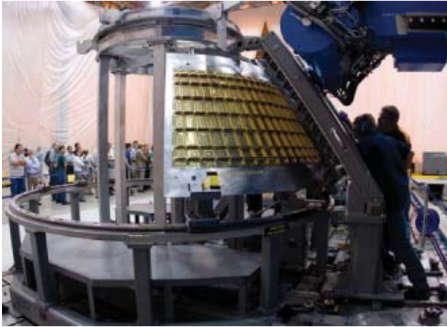
Lockheed Martin weld engineers visually monitor the Universal Weld System II weld head as it completes the five-minute initial Orion friction stir weld. (Photos courtesy of Lockheed Martin.)
