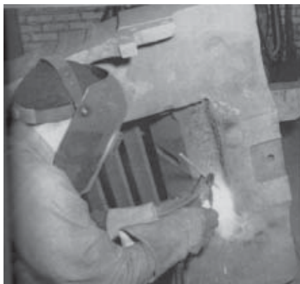
Fig. 2 — As a last resort, air carbon arc cutting was used to salvage this iron casting.
