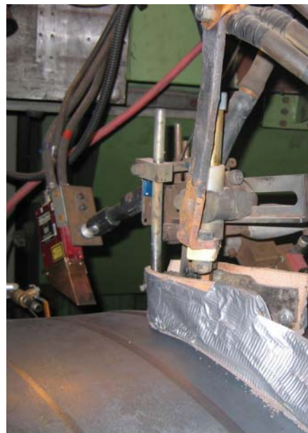
Fig. 2 — Laser vision controlled welding machines in hard and flexible automation.
