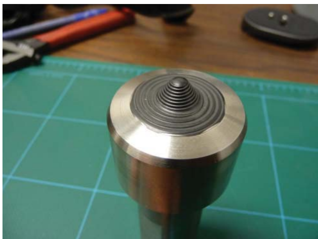
Fig. 4 — A new 6-mm pin tool (left) and one shown after more than 100 ft of weld in A36 steel.
