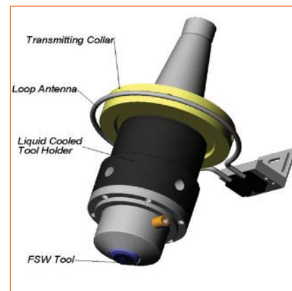
Fig. 3 — An example of the latest tool, tool holder, and telemetry system technology.
