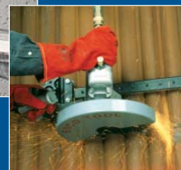
PANELHOG Universal Air Powered Saw cuts panels, removes membrane, and is available with WrapTrack™ kits for cutting pipe from 6" to 60" O.D.
