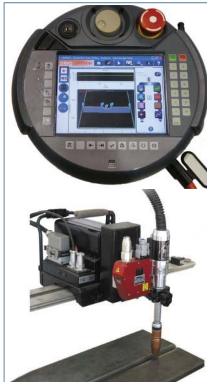
Fig. 6 — Portable welding robot with intelligent interactive teaching method.
