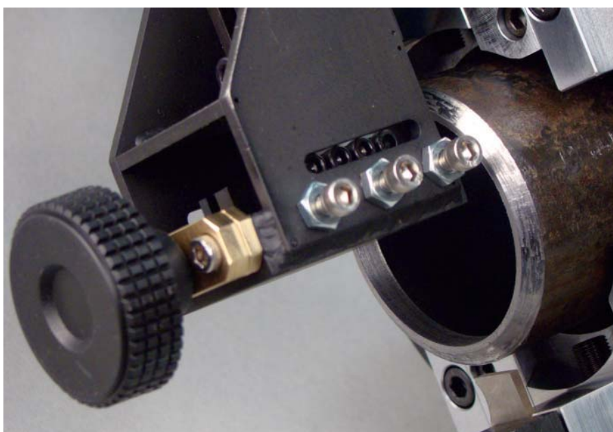
Fig. 1 — Accessories are available as part of a complete machining system. Shown here is a counterbore module machining the inside surface of the weld prep area.
