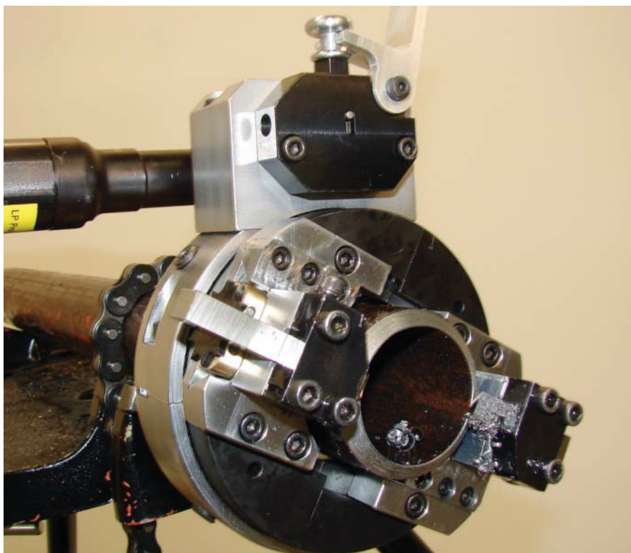
Fig. 2 — OD-mounted split frame machine tool with air drive shown simultaneously parting (cutting) and beveling a standard 37.5-deg weld prep. Note the lathe-quality finish ready for welding.
