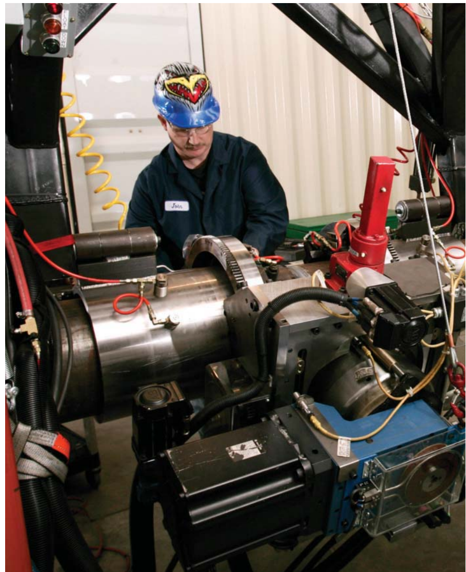
Fig. 7 — An operator sets up the orbital FSW machine.
