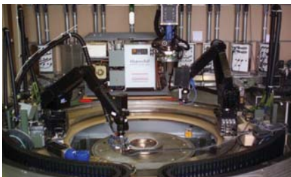
Fig. 4 — Overview of the automated welding system. (Photo courtesy of INL.)
