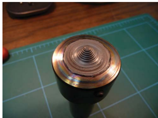
Fig. 4 — A new 6-mm pin tool (left) and one shown after more than 100 ft of weld in A36 steel.
