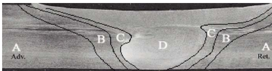
Fig. 5 — Microstructural regions of a friction stir weld: A — Unaffected base metal; B — heat-affected zone (HAZ); C — thermal mechanically affected zone (TMAZ); D — stir zone (SZ).
