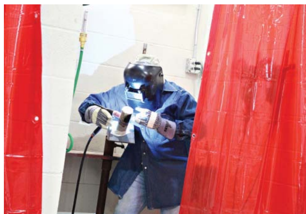
A Zachry Academy welding student tests on 2-in. Schedule 10 (0.109-in.-wall) stainless steel pipe coupons with gas tungsten arc welding using ER-308 filler metal in the 6G position with argon purge and shielding gas.
