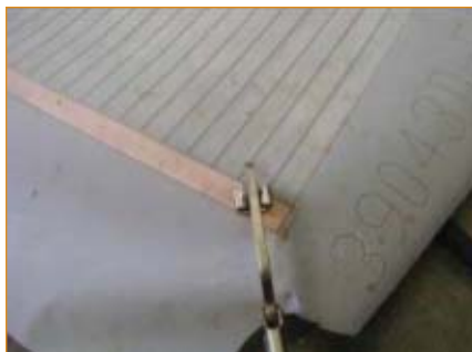
Fig. 9 — Vellum used to fit tubes and extrusions.
