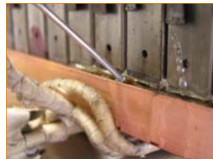
Fig. 12 — Coil providing heat for soldering.
