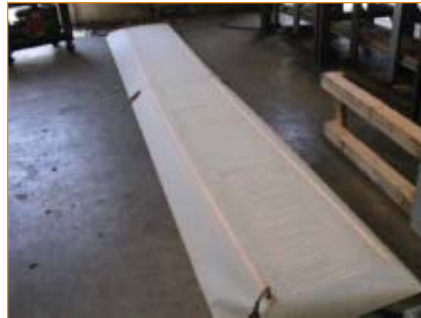
Fig. 16 — Full-size vellum used to check finished track dimensions.
