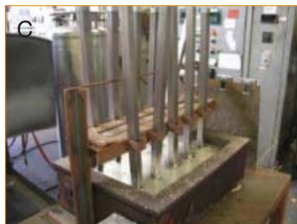
Fig. 6 — A — Preheat; B — fluxing, solder; C — pot immersion; and D — final tinned appearance.
