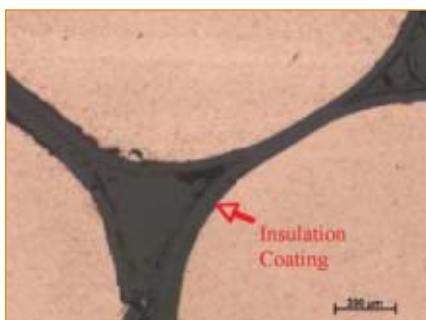
Fig. 5 — Low (top) and higher (bottom) magnification cross-sectional views through the Litz wire inside bar.
