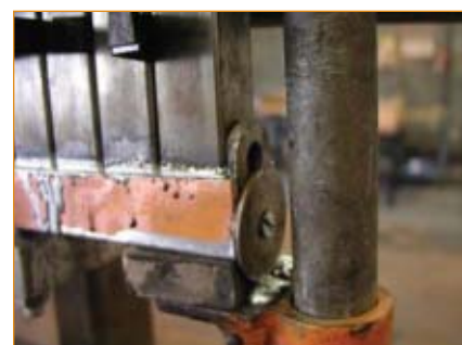
Fig. 13 — Dam used to control solder flow.
