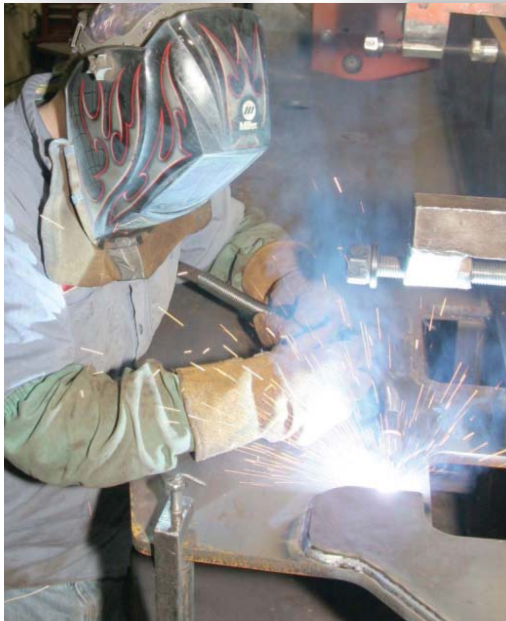
The condition of the material being welded, plus its postweld requirements, both contribute to filler metal selection.
