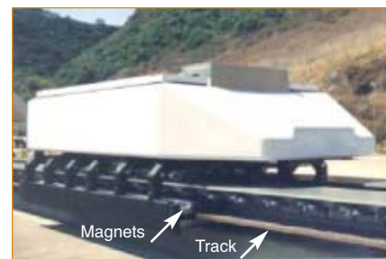
Fig. 1 — Conceptual and demonstration vehicles and track/magnet relationship.
