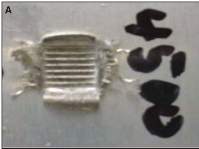
Fig. 7 — Part marking. A — Without, and B — with Cu buffer sheets.
