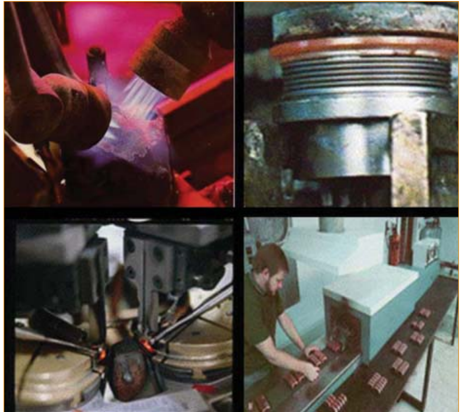
Fig. 3 — The main brazing heating methods are (clockwise from top-left) torch, induction, furnace, and resistance.
