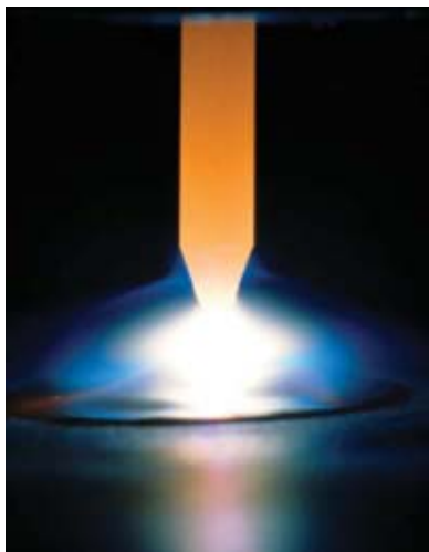
Fig. 1 — The GTAW process using AC current to produce an arc between a tungsten electrode and the aluminum plate and protecting the molten aluminum with pure argon shielding gas. (Reproduced by permission, TWI Ltd.)
