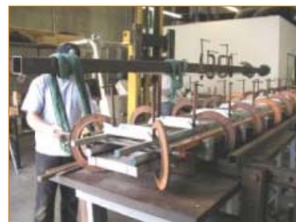
Fig. 8 — Fixture used to set up Litz bars and extrusions.
