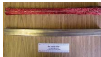
Fig. 3 — Litz wire (top) removed from bar and stainless steel bar enclosure (bottom).
