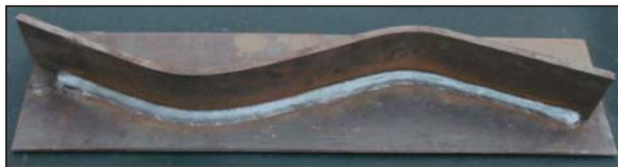
Fig. 24 — Result of tracking a curved weld joint.
