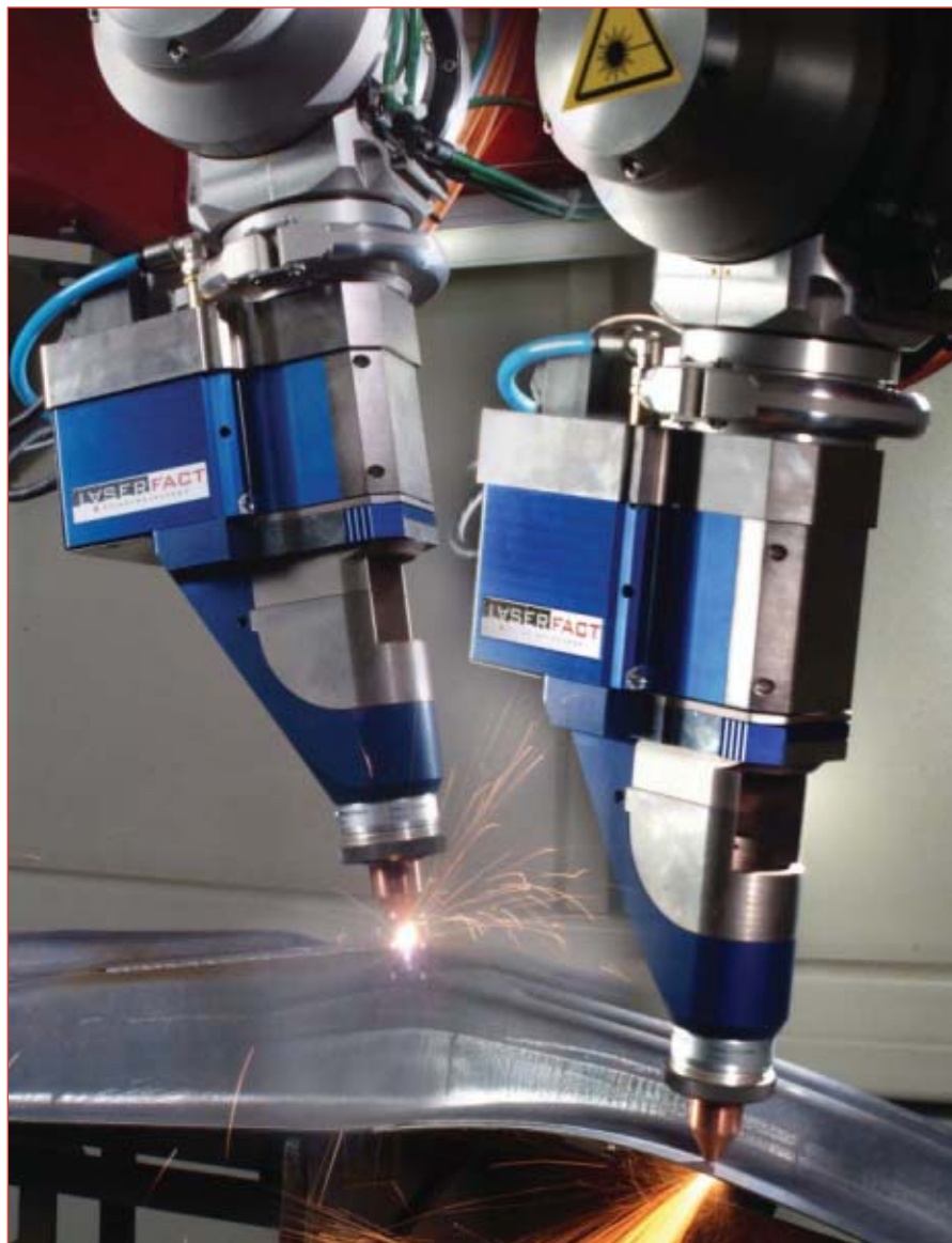
Fig. 6 — Combi-head at work. Cutting and welding process on the B-pillar with a gantry robot. (Photo courtesy of Laserfact GmbH.)
