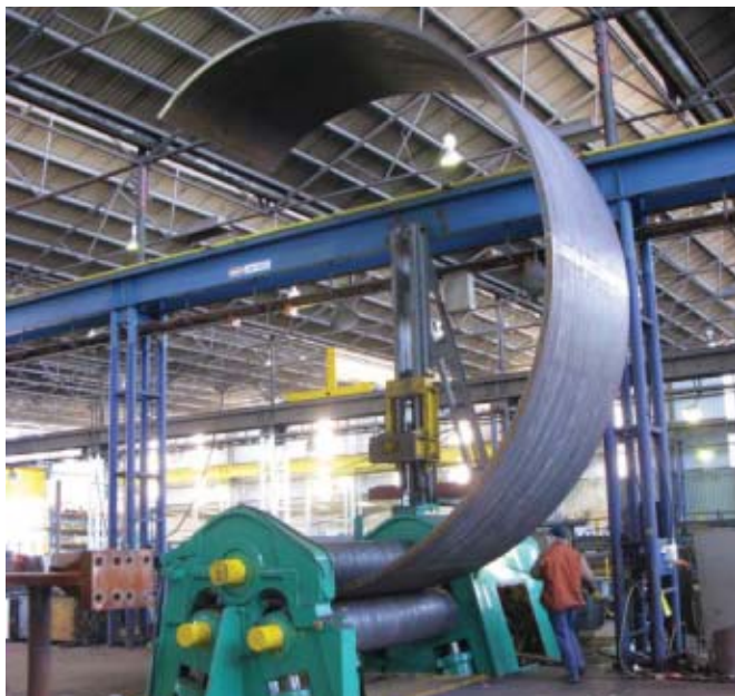
Fig. 1 — Prior to submerged arc welding, 14.5-m-long steel sheets were cut and rolled into cylinders.
