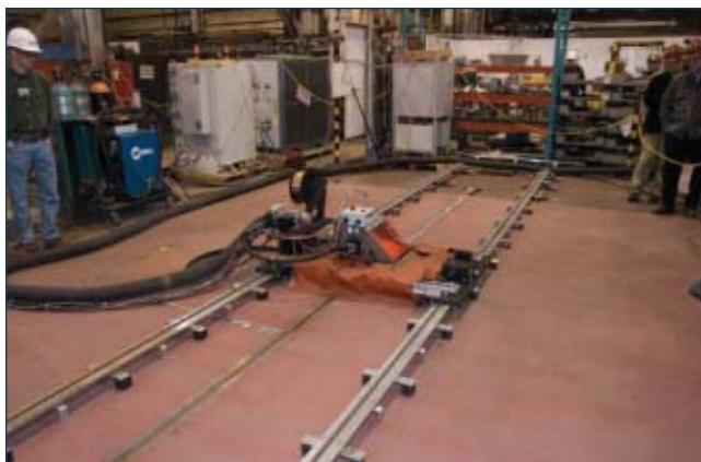
Fig. 3 — Hybrid laser arc welding demonstration system joining two 20-ft panel sections at Bath Iron Works in January 2008.
