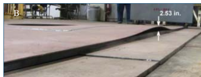
Fig. 5 — A — HLAW and B — SAW demonstration panels comparing the magnitude of out-of-plane distortion adjacent to the insert after welding. The out-of-plane deflection from a flat position is indicated (the value includes the plate thickness).
