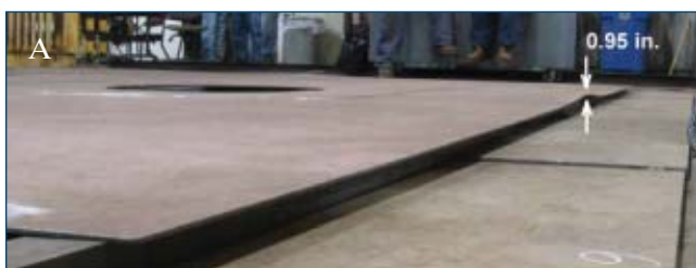
Fig. 5 — A — HLAW and B — SAW demonstration panels comparing the magnitude of out-of-plane distortion adjacent to the insert after welding. The out-of-plane deflection from a flat position is indicated (the value includes the plate thickness).
