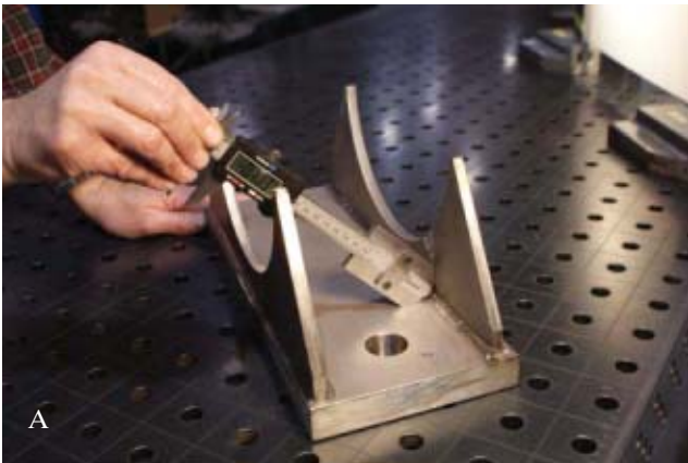
Fig. 3 — A — When touching the weld face, the digital scale shows the actual distance from the root to the face, providing a measurement of the actual weld throat; B — a close-up of the throat measurement.
