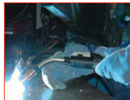
Fig. 9 — The HD Q™ and S™ series guns come in 300- to 600-A models designed for high-deposition GMAW applications.
