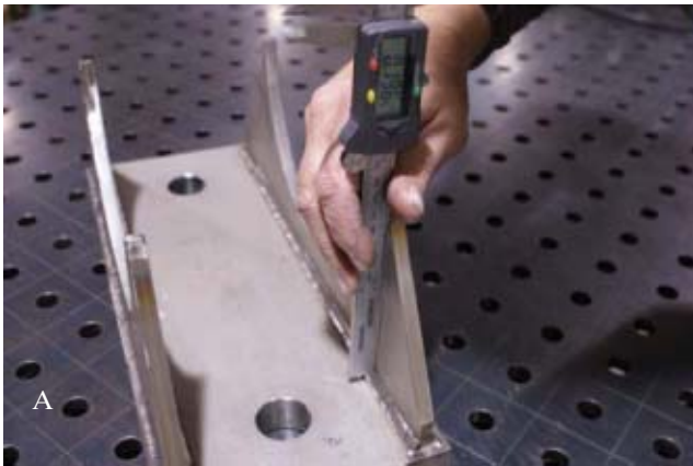
Fig. 4 — A — A similar technique, using a traditional caliper, is used to measure the leg length; B — a close-up of the leg measurement.
