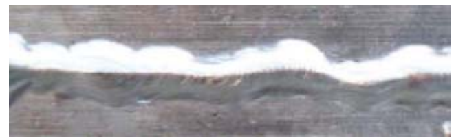
Fig. 8 — Example of typical GMA weld bead in Ti-6Al-4V without IPQA.
