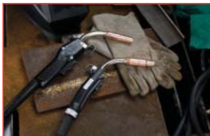
Fig. 6 — Shown are two GMA guns (from left) Number 4 along with the Spray Master™ 450 model that handles heavy-duty, pulse, and spray applications.
