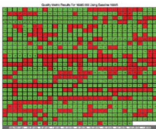
Fig. 7 — Quality metric matrix corresponding to a LFW undercut condition.
