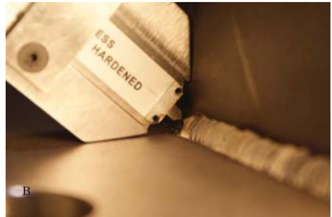
Fig. 3 — A — When touching the weld face, the digital scale shows the actual distance from the root to the face, providing a measurement of the actual weld throat; B — a close-up of the throat measurement.
