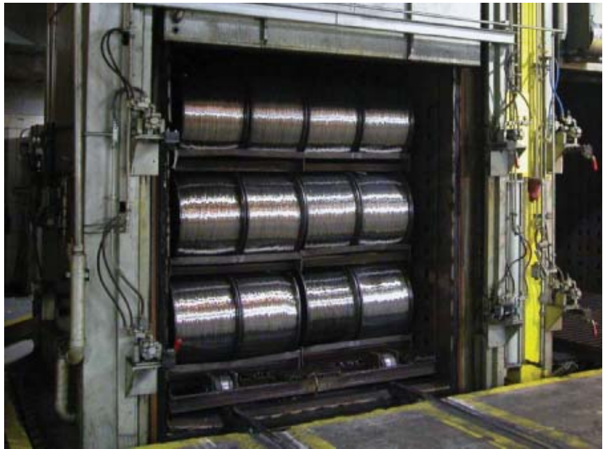
Fig. 1 — These 600-lb spools of aluminum welding wire are about to undergo an annealing operation to remove the work hardening effect produced by previous wire drawing operations.
