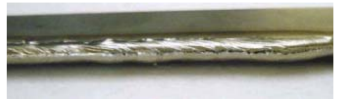
Fig. 9 — Example of typical GMA weld bead in Ti-6Al-4V with IPQA.
