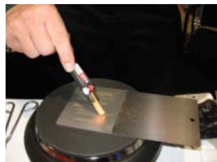
Fig. 12 — Stroke the workpiece during heating, and Tempilstik-Pro™ will make a distinct mark by melting at the point of contact once the surface reaches the product's rated temperature.
