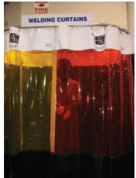
Fig. 8 — Running on a steel track and roller system for easy gliding, Curtain Walls™ use Velcro® to make taking apart and putting them together simple.
