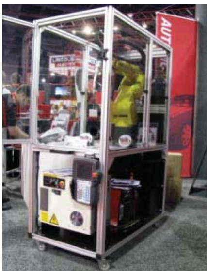
Fig. 13 — This small-sized robot welding cell can be wheeled from one classroom to another to train students about robot programming.
