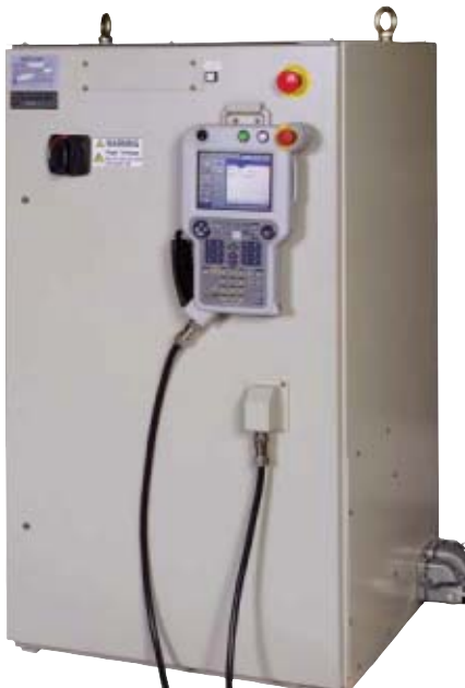
Fig. 6 — The NX100 robot controller is capable of handling up to four robots.
