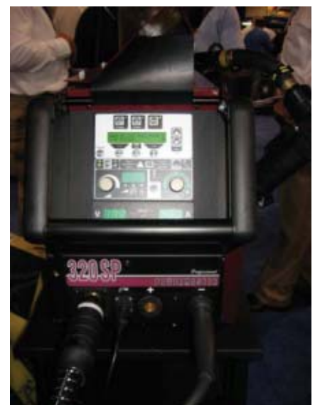
Fig. 9 — The PowerMaster® 320SP is portable and welds nonferrous materials up to 1/4-in. plate.
