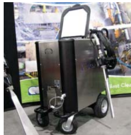
Fig. 16 — The Aero 80-DX dry ice blast cleaning system from Cold Jet offers a blast pressure range of 30–140 lb/in. 2 for aggressive cleaning action.
