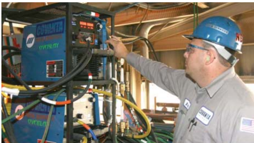
Fig. 3 — Brad Hooper walks through the four-step setup for setting pulsed GMAW parameters on the XMT 350 MPA. The units retain settings for each process, so they can easily be switched from GMAW-P to SMAW and back with a simple turn of the knob.
